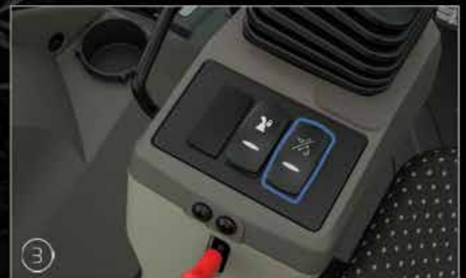
Shifter Button for Backhoe or Loader Function
