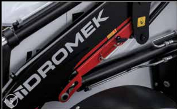
⑤ Loader boom support device
