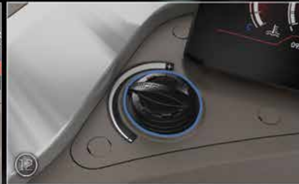
Hand Throttle with Electronic Rotary Control (*)
