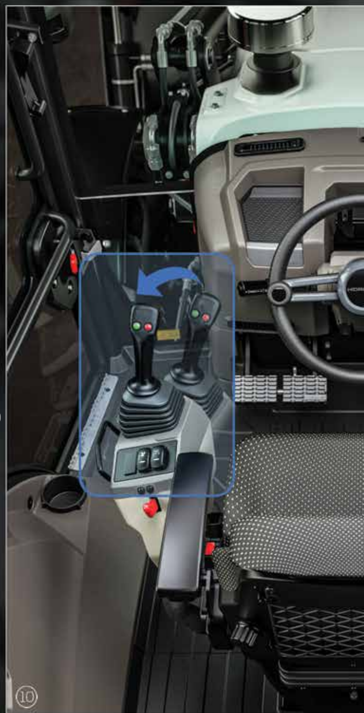
⑩ Tilting of the left joystick to some extent for the operator to work more comfortably on the loader side
